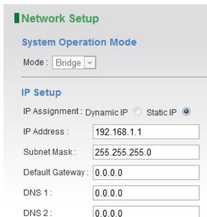
The screenshot shows the 'Network Setup' configuration page. Under 'System Operation Mode', the 'Mode' is set to 'Bridge'. The 'IP Setup' section has 'IP Assignment' set to 'Dynamic IP' (selected with a radio button) and 'Static IP' (unselected). Below this are input fields for 'IP Address' (192.168.1.1), 'Subnet Mask' (255.255.255.0), 'Default Gateway' (0.0.0.0), 'DNS 1' (0.0.0.0), and 'DNS 2' (0.0.0.0).
