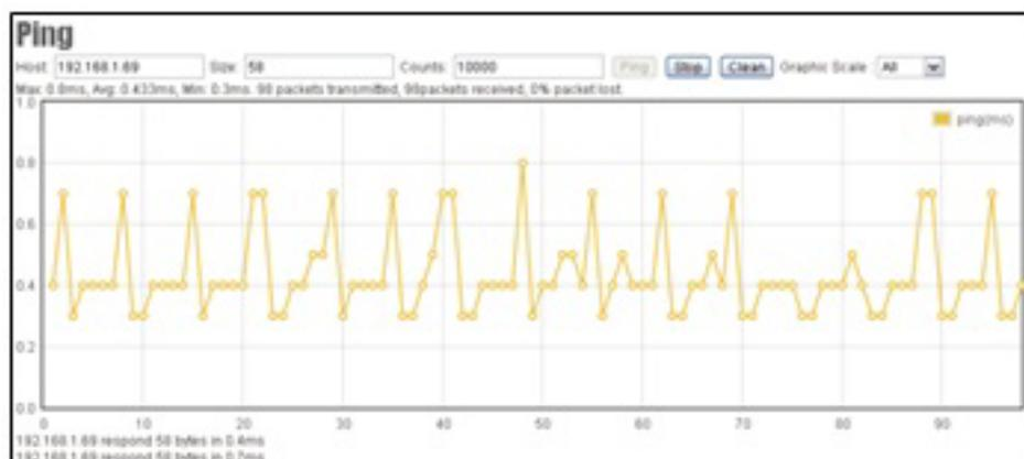
Graphical display helps administrator to get the responding time changes of target IP address. Insert the remote host IP address, packet size and number in field then press Ping, system will show the results on page. The result presenting can be adjusted by different choosing of graphic scale.
