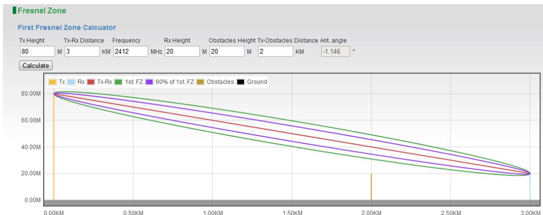
The First Fresnel Zone Calculator is a tool that helps you to estimate the possible obstruction from existing object between two devices before the wireless installation. An antenna angle calculation can also help you to aligning the vertical angle of the directional antenna.
