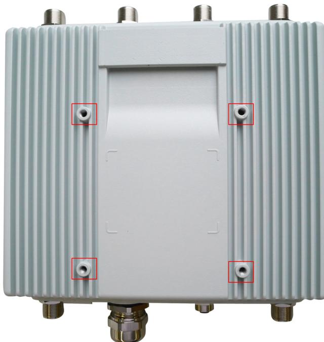
2. Fix the wall mounting plate onto back side of EKI-6340 as below:
