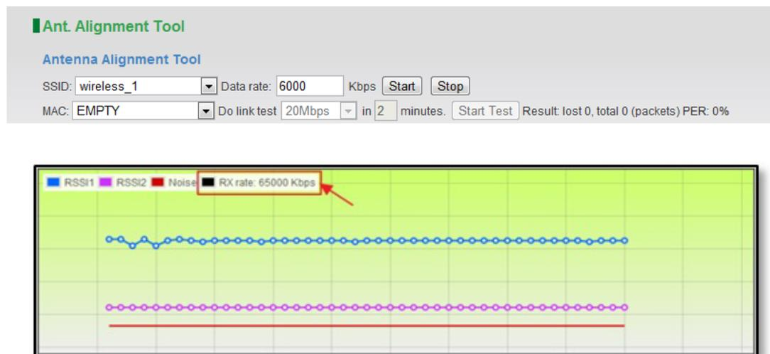
An Rx rate shows the best data rate you can reach under the current RSSI level. Link Test Tool can also help you to do the fine tuning of your antenna direction.
