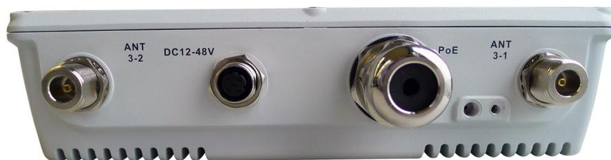
Figure 2.3 Bottom view of data port & power port of Advantech EKI-6340
