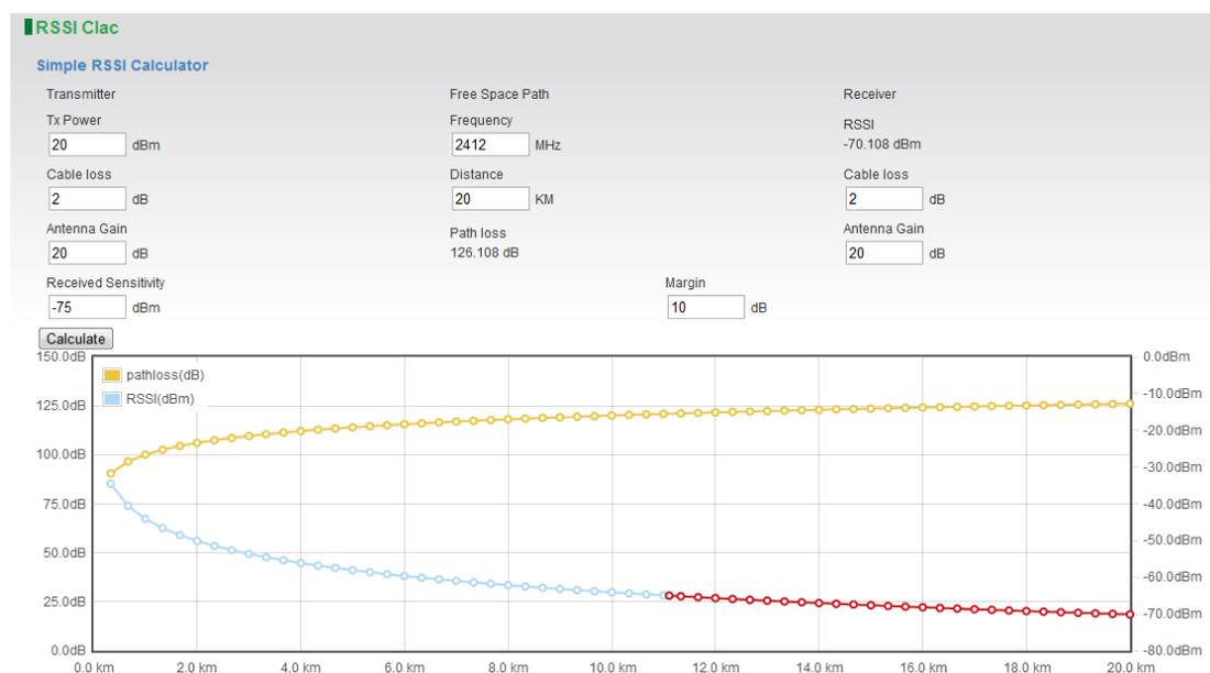
Simple RSSI Calculator helps to estimate a possible RSSI and path loss by known device's Tx power (transmission power), cable loss, antenna gain and frequency on both transmitting and receiving sides. Graphic displaying shows changes of path loss and RSSI.
