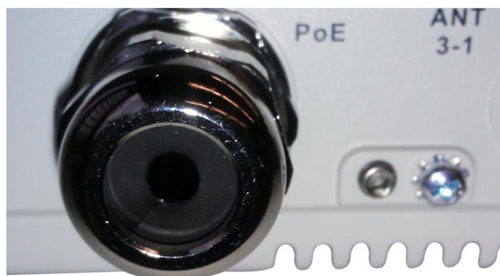
2. Pass Ethernet cable through M25 cable gland.
