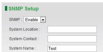
EKI-6340 series supports both SNMP V2 and V3. The configurable items show below:
