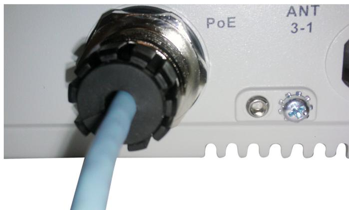
4. Fasten the cable gland cover to ensure the waterproof function of PoE port.
