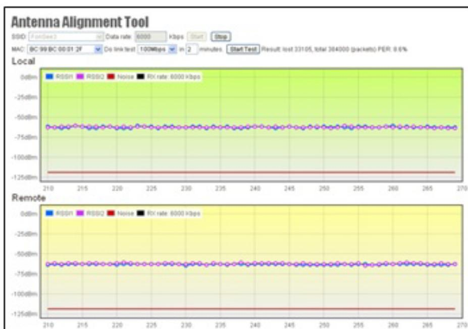
Choose the SSID which you are going to do the antenna aligning and click the Start button both access point and wireless station (AP Client) side to start the antenna alignment. You will be able to see the RSSI changes in figure. Try to adjust the directional antenna's horizontal and vertical angle to get the best RSSI level.
